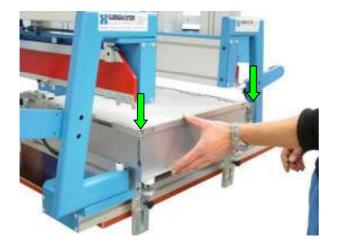
Attach the rear panel of the drawer and press it with both hands laterally and from above respectively onto the adapter hooks till it locks into place.
