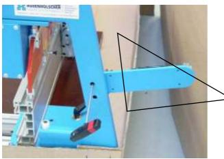
Swing in the side panel cylinder 90° and mount it with the screws supplied. Perform the procedure for both side panel cylinders.
