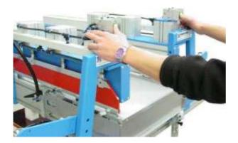
Press the two-hand control device and the drawer parts will be assembled.
