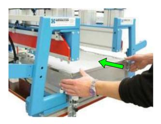
Move the rear panel together with the side panels against the positive stop.
