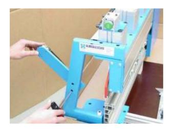
Mounting of the side panel cylinder Loosen the bottom screw
