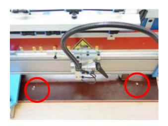
The assembly unit is fastened on the base plate to the transport palette with screws (see pictures).
