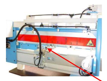
Setting of the drawer depth Pull up the indexing bolt, adjust to the size wanted and lock into place!
