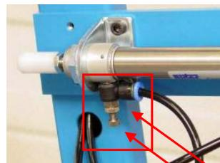
In order to assure smooth operation of the drawer assembly the side panel cylinders have to put up the side panels against the bottom of the drawer at the same time. The adjustment for simultaneous extension of the cylinders can be done with a throttle.
