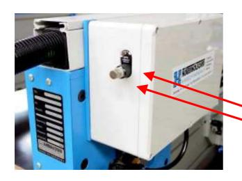
Factory setting (0.15 – 0.20 bar) for the counter pressure of the side panels.
